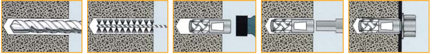
Drill to recommended depth. Clean hole thoroughly with brush & blow clean. Insert anchor with hammer. Expand anchor using setting tool. Set anchor with bolt.
