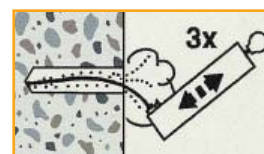
2. Clean the hole as shown using stiff wire or nylon brush and compressed air or dust blower.
