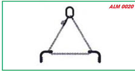
Case grab sling with shortening clutch
